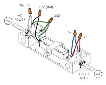
\* LED Driver and J-Box must be grounded in accordance with local and national electrical codes. Ground the LED Driver and J-Box with the included Green Grounding Screw. Some compatible LED drivers are Class II certified and do not require a FG (Fault Ground Connection). Refer to the LED driver label and installation guide for more information.
